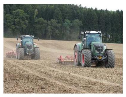
Fendt GuideConnect: Two tractors, one driver RTK-guided autosteer + V2V wireless communication
