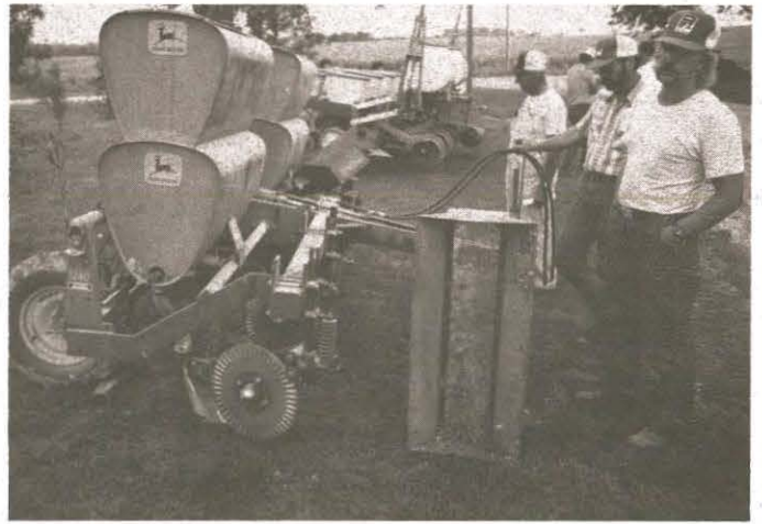
A shop-crafted rig for applying dry fertilizer, shown at the field day of Mark and Rita Mays, Wilton. The screen, standing upright, is used in filling the hoppers.
