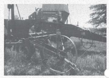
Electronically activated relays drop several seeds per hill. On this prototype, a paddle wheel drives the circuitry and synchronizes the planter with the previous pass.
