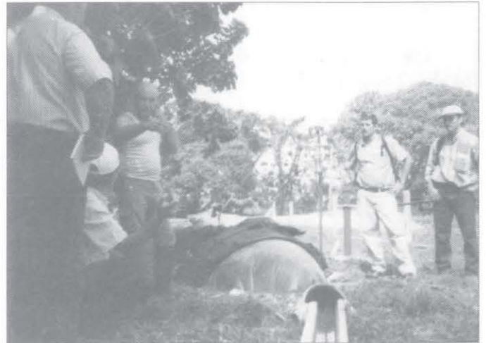
This bag digester turns swine waste into biogas for cooking on the farm of Ernesto González (facing, left).
