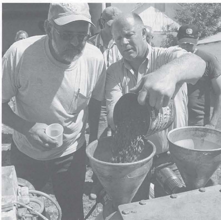
Gary Laydon watches as Kim Odden feeds the dual-expeller press, capable of 50 gallons in 24 hours.
