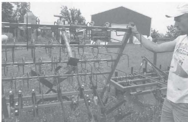
The Lely tines on the Williams Tine Weeder flip up and down quickly and easily to accommodate different plantings
