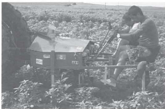
Operators guide the spinning discs of the Reigi to remove weeds
