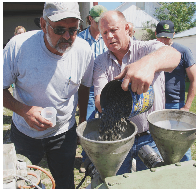
Gary Laydon watches as Kim Odden feeds the dual-exPELLER press, capable of 50 gallons in 24 hours.
