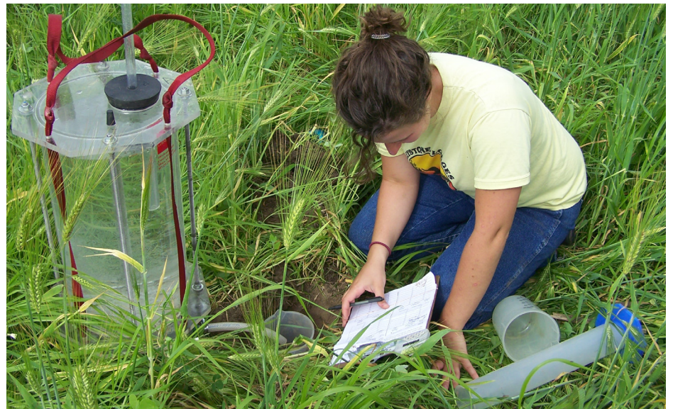
Kayla Koether recording steady-state, water-infiltration-rate data using a Cornell sprinkle infiltrometer.
