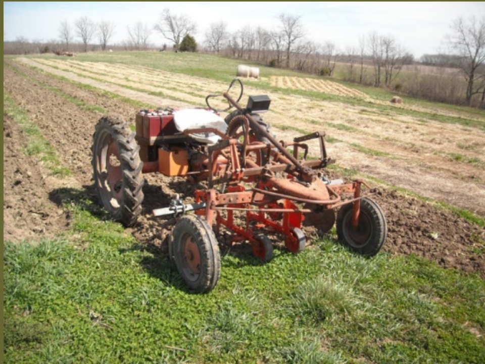
1947 Allis Chalmers G with electric conversion
