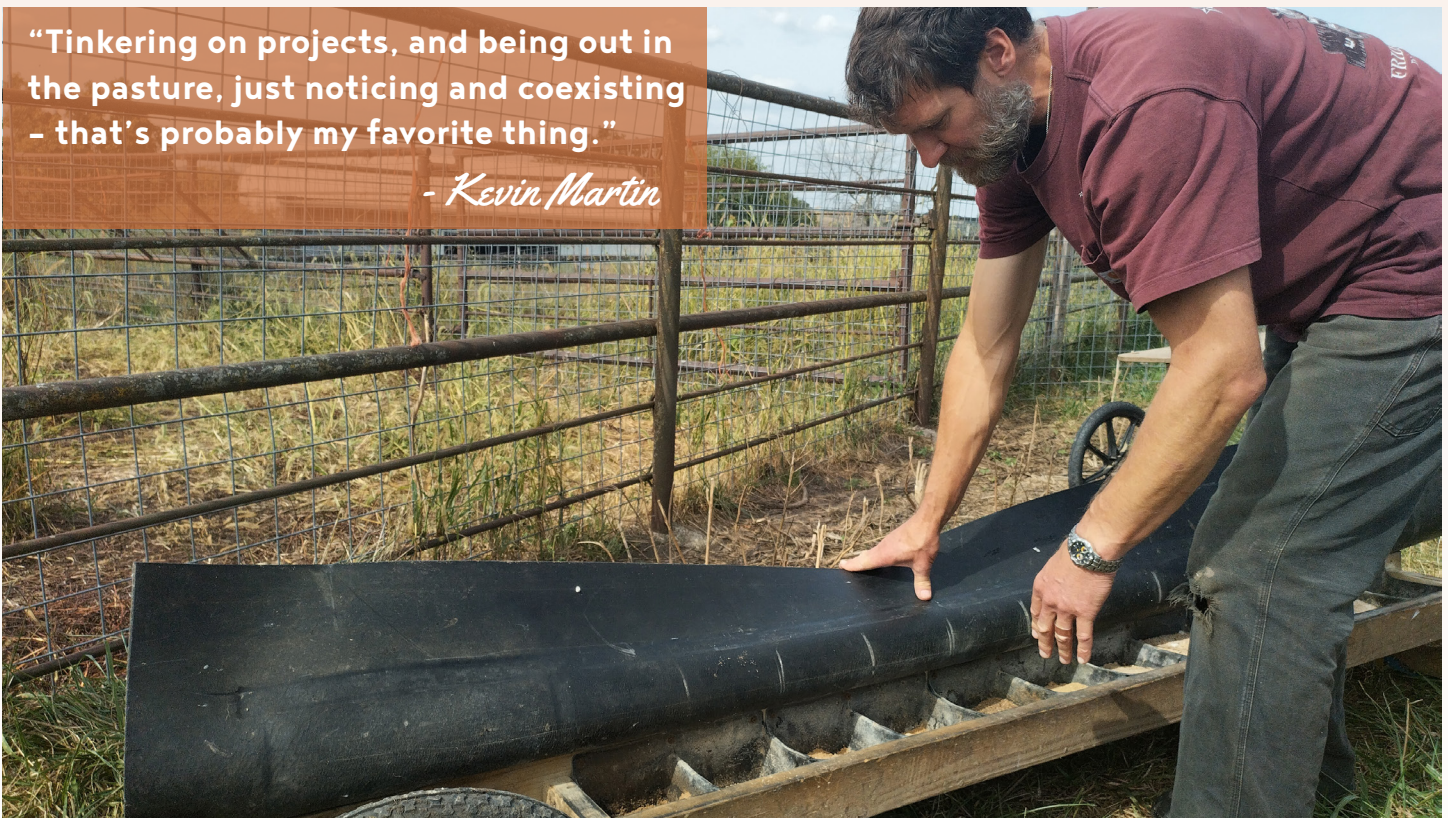
Kevin points out the rubber lid on a early mineral feeder design. Though weatherproof, the goats liked to stand on it too much.
