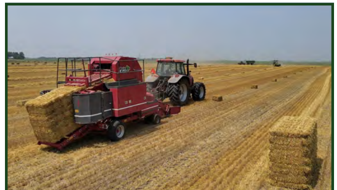
Left: The winners of the 'baling party' gather on the Knuth's farm. Right: The Bale Baron, a machine that accumulates small square bales in packs of 21, which makes for streamlined transportation.
