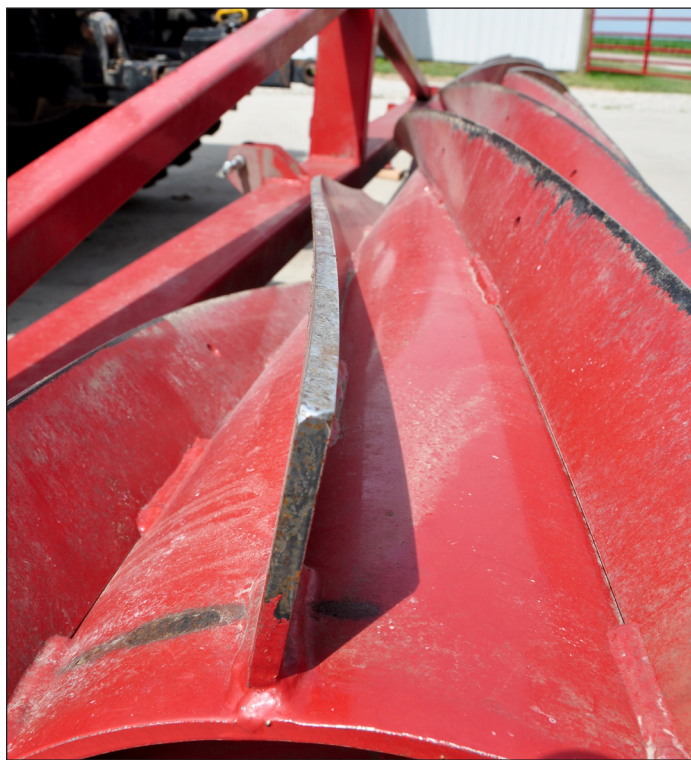
The Chevron-pattern on the crimper roller prevents soil disturbance and reduces vibration in the tractor. The blunt edges snap the rye stem without cutting it.
